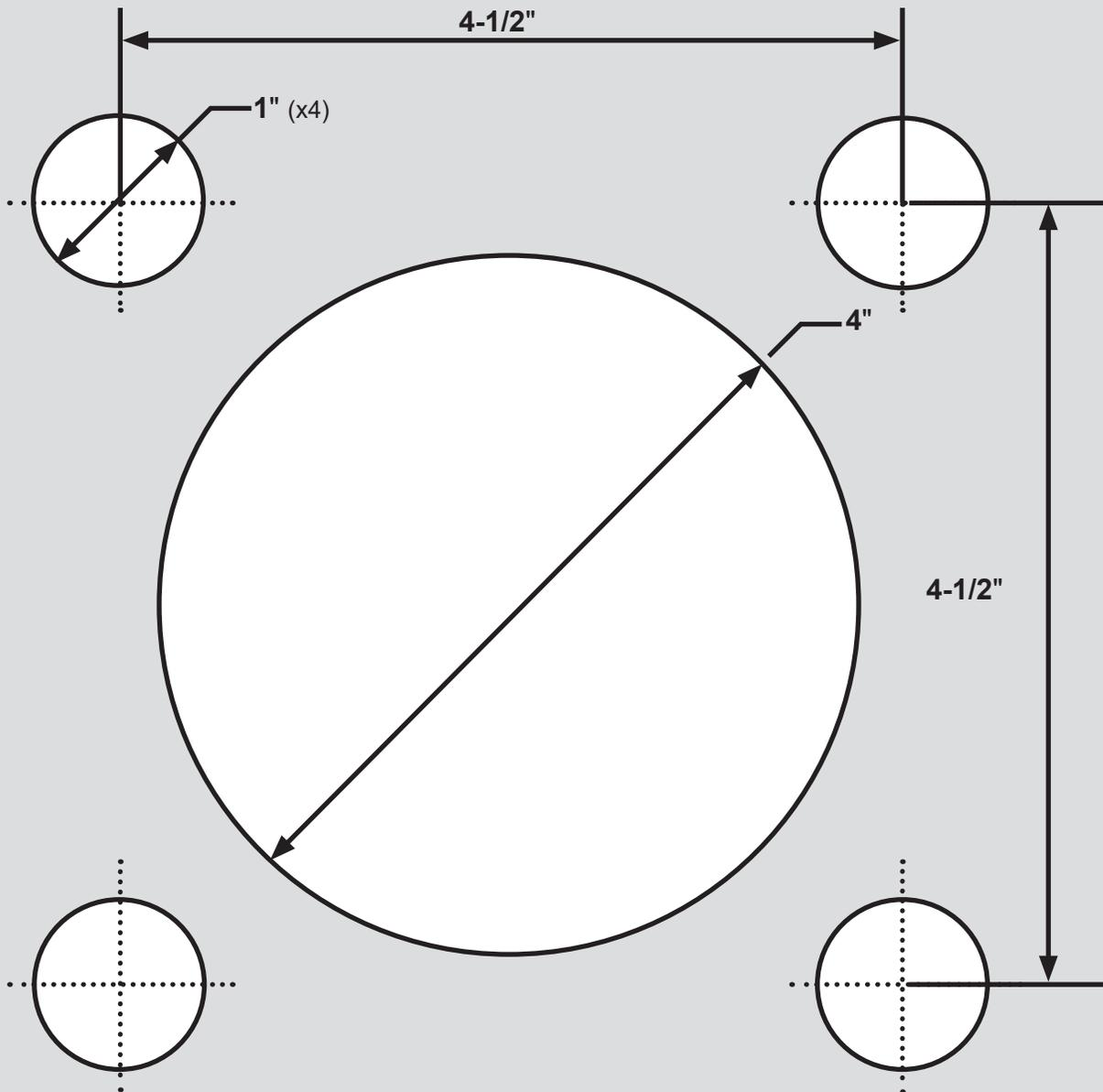
**NOTE:** It is recommended to transfer this template to a piece of wood (1/2" to 1" thickness) to ensure proper anchor bolt placement.
