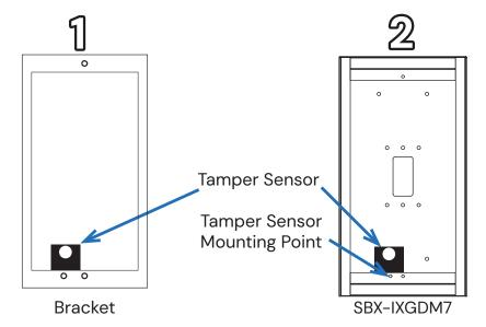
Thread all wires through the chosen wire passthrough or conduit knockout and mount the SBX-IXGDM7 to the wall. Attach all wires to the IX-DM7-HIDA. Insert the IXG-DM7-HIDA into the SBX-IXGDM7 and insert and tighten the mounting screws.
