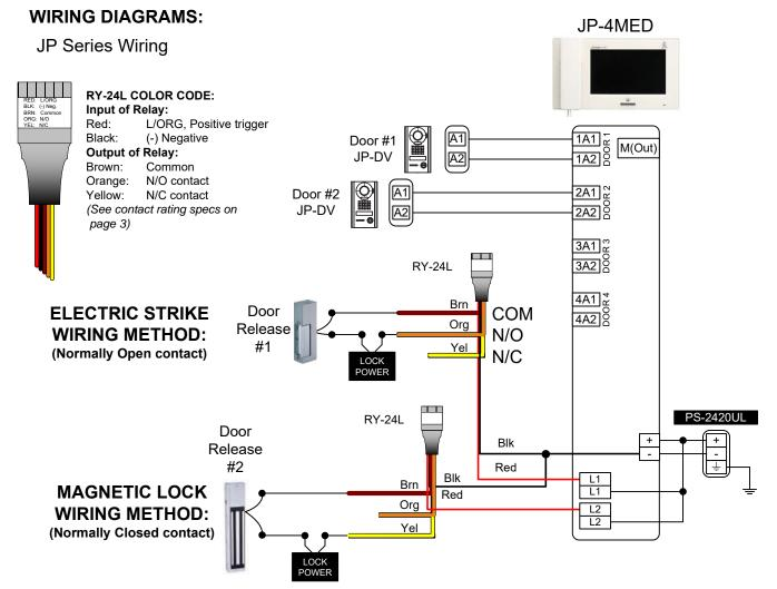
NOTE: The door release contacts on the station are rated at 24V AC, 500mA. The RY-24L should be used in any application where the strike or maglock has a higher voltage or draws more current. Otherwise, internal damage to the master station could occur.
