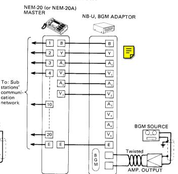
NOTE: Remove jumper between  $\boxed{A1}$  and  $\boxed{V1}$  on master station.
