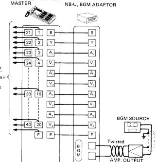
NOTE: Remove jumper between  $\boxed{A1}$  and  $\boxed{V1}$ ,  $\boxed{A2}$  and  $\boxed{V2}$ ,  $\boxed{A3}$  and  $\boxed{V3}$ ,  $\boxed{A4}$  and  $\boxed{V4}$  on master station.
