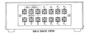
BGM : Connect to output terminals of the amplifier.
