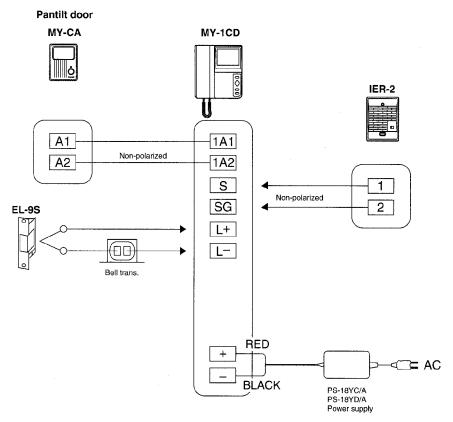
MY-1CD can be powered by a power supply PS-18YC/A (AC 120V) or PS-18YD/A (AC 220-240V). When PS-18YC or PS-18YD is used, plug in to DC receptacle provided on back of MY-1CD.
