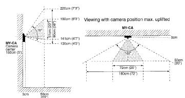
Pantilt camera vision at 50 cm (20") distance (vertical x horizontal)
