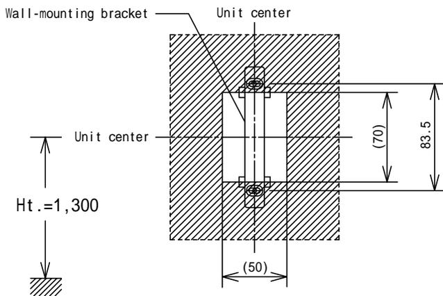
Cable inlet opening; As provided for single-gang mounting
