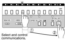
A call is announced by both electronic mono tone and LED. Depress a selector button below the illuminated LED. Depress TALK button to talk, and release to listen. After communication, depress OFF button.
