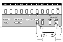
Depress ALL CALL button. The all call mode indicator LED is lit. Depress TALK button while making announcement. After announcement, release ALL CALL button by depressing the button again.
