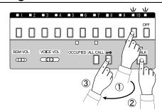
Door station call-in is announced by electronic mono tone and the image of a caller appears on all video monitors. Depress a selector button below the illuminated LED. Depress TALK button to talk and release to listen.
