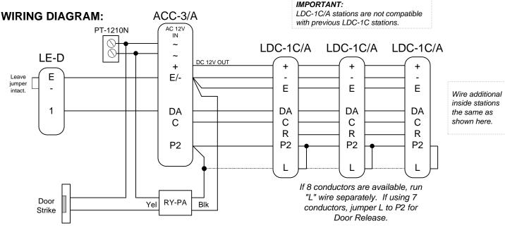
LDC-S: DOOR COM SET, includes 3 LDC-1C/A Inside Stations, 1 LE-D Door Station, 1 ACC-3/A Adaptor, and 1 PT-1210N Transformer.
