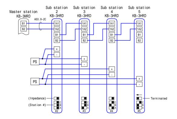
Observe that each two Sub stations (#1 & 2, and #3 & 4) are powered by a separate Power supply. (KB-3MRD Master station is always powered by a single Power supply, not combined with Sub stations).
