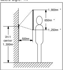
Camera angle: -7  $^{\circ}$  (When the station is at a high position due to a step)
