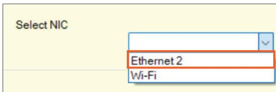
Make sure that the network information assigned to the IX-SOFT instance matches its new PC. Consult the site's network administrator to see what information should be used. Once that is established, navigate to **Network Settings**, *IP Address* on the left hand menu. If the IP address or subnet mask for IX-SOFT needs to be adjusted, make the change in the appropriate cells and click **Update**.
