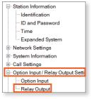
Under [Display Settings], select Relay Output 2. Remove the checkmarks for the door station under <u>Status Output 2</u>, <u>Outgoing Call</u>. Click **Update**.
