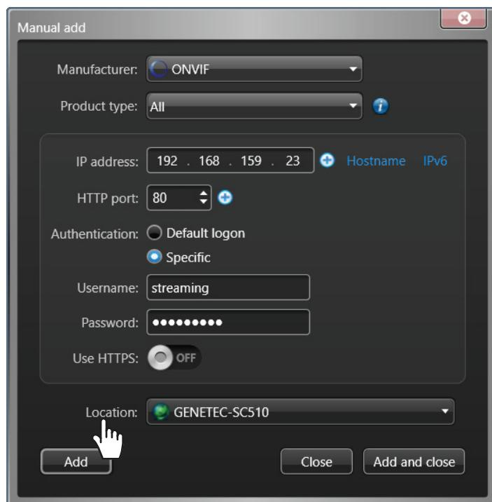
To add a door or entrance station to the system, fill in the IP address, ONVIF ID, and password. Set the HTTP port to 80 and the manufacturer to ONVIF. Click **Add**. Repeat the steps for each IXG-DM7-HIDA and door station that will stream video to Genetec.
