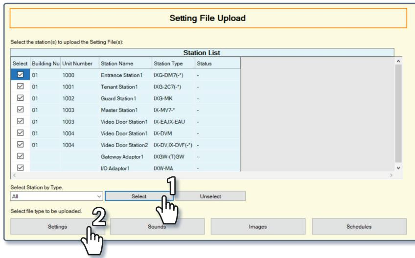
**i** If a station upload fails, make sure that the programming PC is in the same IP range as the stations.
