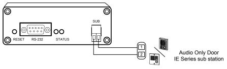
\* Wiring to sub station should be 2-conductor shielded cable. Wire distance from IPW-1A to IE series sub station: 22AWG = 387 feet. 18AWG = 980 feet
