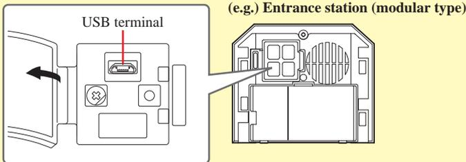
NOTE: Set the "COM Port" setting to the USB terminal number that is used for connecting to GT-BCXB-N. ( → [7-1](#) )
