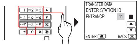
During transfer, "TRANSFERRING..." is displayed and the IN USE LED stays lit.
