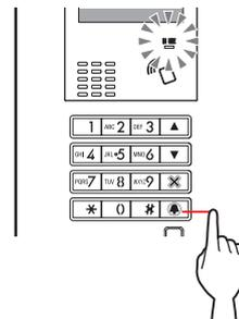
The IN USE LED will flash, and then change to being lit to show that the unit has entered into the programming mode.
