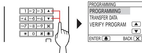
7 Press **ENTER**, and wait until the IN USE LED changes from flashing to staying lit.
