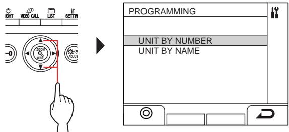
**16** Display the assigned unit by using the 10-key, then press
