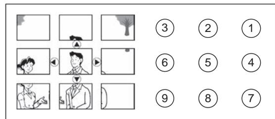
**Setting method:** Select the desired position number ① to ⑨ by using the 10-key.
