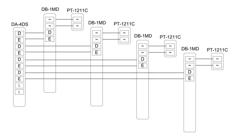
L and L terminals on the door station provide 15vac for door release strike.
