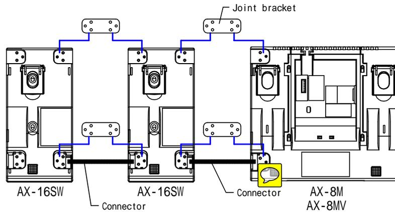
Interconnect Master station & AX-16SW units, plugging the supplied CAT5e cable connector in each socket.
