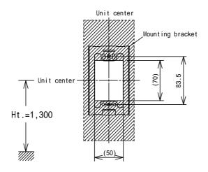
Cable inlet opening: Provided for single-gang mounting
