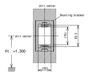
Cable inlet opening; Provided for single-gang mounting
