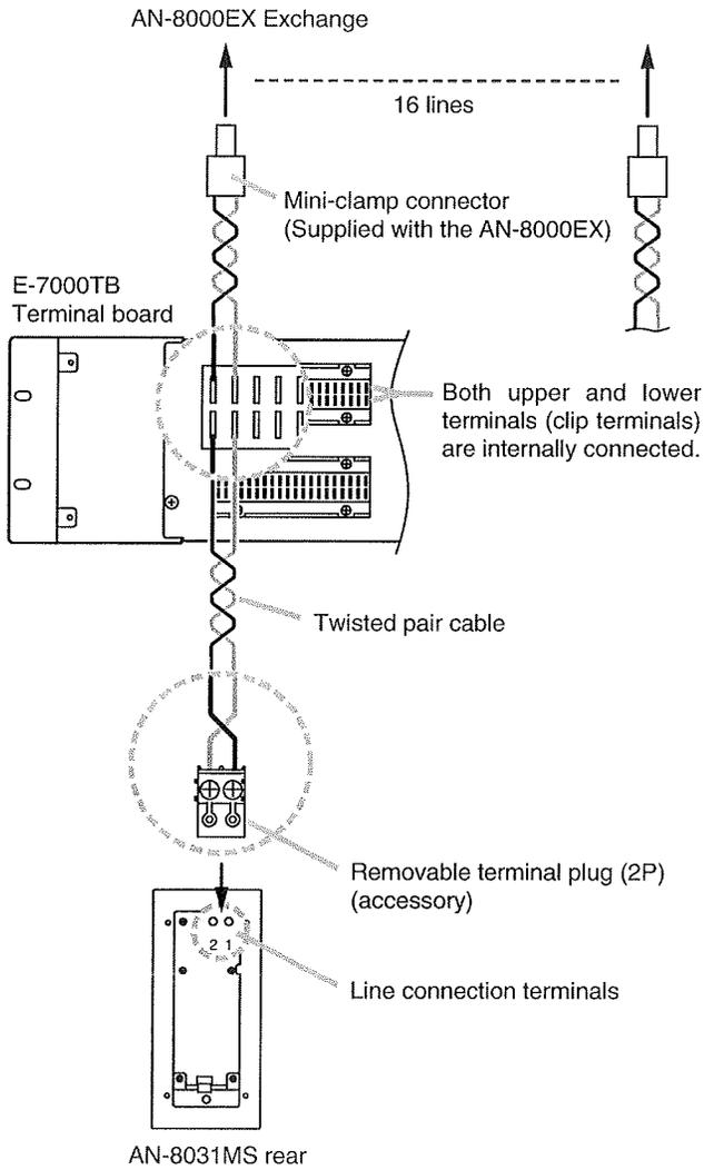
To connect the cables from the AN-8000EX Exchange to the AN-8031MS, use the removable terminal plug (2P) supplied with the AN-8031MS. The cables have no polarity.
