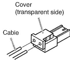
**Step 2.** With a pair of pliers, lightly pinch the mini-clamp cover and, after ensuring that the cable is securely inserted, firmly squeeze on the cover.
