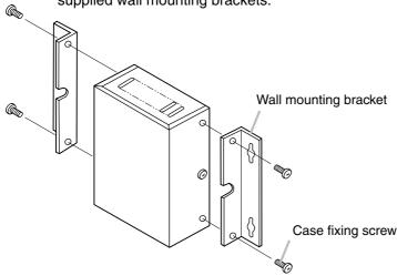
**Step 2.** Fix the unit on the wall. Use the supplied wood screws (3.5 x 25) as appropriate for mounting.
