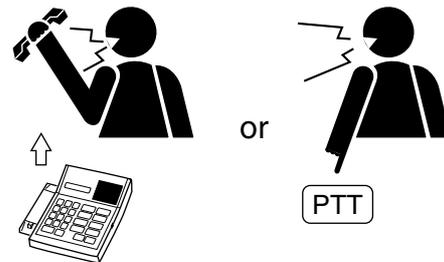
**Step 3.** To terminate the conversation, replace the handset or press the [C] key.
