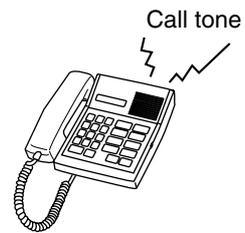
**Step 2.** Lifting the handset stops the call tone and permits conversation to proceed. (A response can also be made by pressing the [PTT] key for handsfree conversation.)
