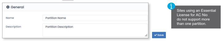
To create a new partition, navigate back to **System**, <u>Partitions</u>. Click the cog wheel next to the default partition to open a new menu. Click <u>+Add</u>. Give the partition a **Name** and **Description**. If **Auto Panel Update** is checked, any panel that is added to the partition will automatically be updated 15 minutes after changes are made. Click <u>+Create</u> to finish adding the partition to AC Nio.
