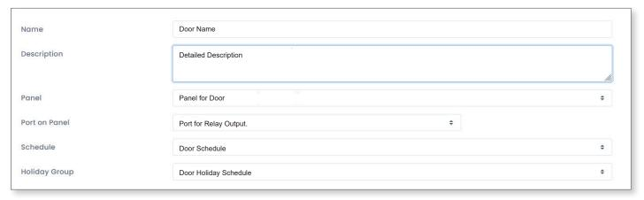
Next, the settings for the reader itself need to be configured. Assign the reader a **Name** and detailed **Description**. Select the Wiegand port the door's card reader will be wired to from in the **Port on Panel** field.
