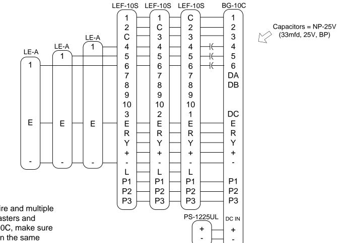
When using a 10 conductor wire and multiple 2 conductor wires between masters and between the master and BG-10C, make sure the # terminal wires (1-6) are in the same jacketed cable as the E terminal wire.
