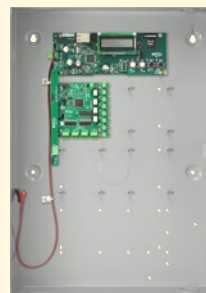
ACS-IO I/O Starter Kit with Enclosure (includes one I/O master controller, one AC-IOE expander board, and one AC-C enclosure, which has space for the required AC-PS1250 power supply— one more AC-PS1250 power supply and up to seven AC-IOE expander boards can be added for a 64-contact capacity) → p. 73
