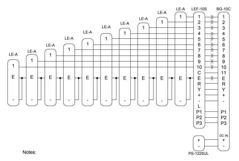
The capacitors used are the NP-25V (33 mfd, 25V, non-polarized). The BG-10C requires the PS-1225UL.
